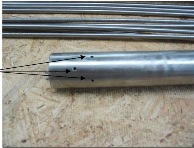
To check for proper assembly, make certain that the impact holes line up with the flag on the opposite end. If they are not, the outer tubes are in the wrong order and this can result in a false null reading.
