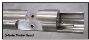
The 5-Hole Velocity Probe is a proven device capable of measuring and correcting angular flow vectors
