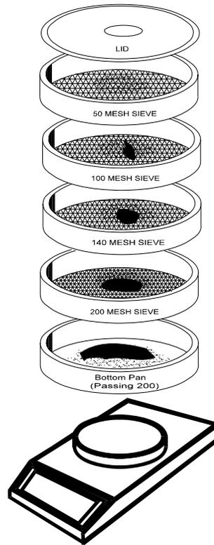
PLACE 50 GRAMS OF COAL ON STACKED 50, 100, 140 AND 200 MESH SIEVES AND SHAKE FOR 20 Minutes
