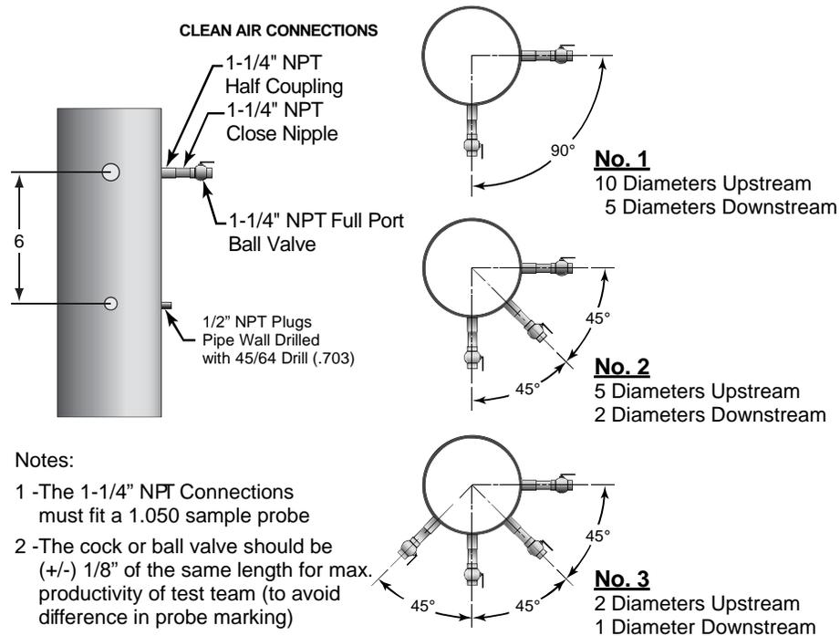
2. Traverse points on the Pitot tube are marked on an equal area grid in accordance to ASME Performance Test Code for traversing circular ducts. This ASME standard, for pipes with 10" or larger diameters, is illustrated by Figure 2.
