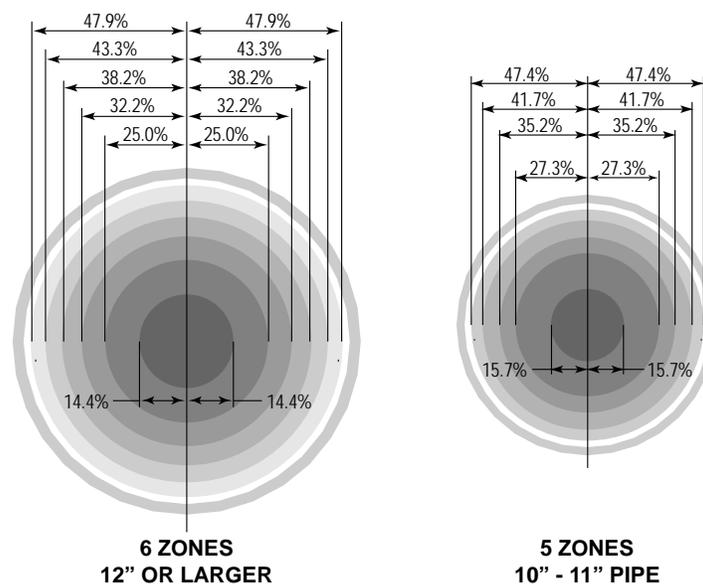
**EQUAL AREA TRAVERSE GRID FOR CIRCULAR DUCTS AND PIPE
