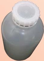
The glass sampling jar that is so easily broken on the older samplers has been replaced with a **high density plastic jug**. The jug has mason jar threads for quick emptying of the collected sample, an O-ring to prevent leakage and its one gallon size is large enough to handle any sampling job.
